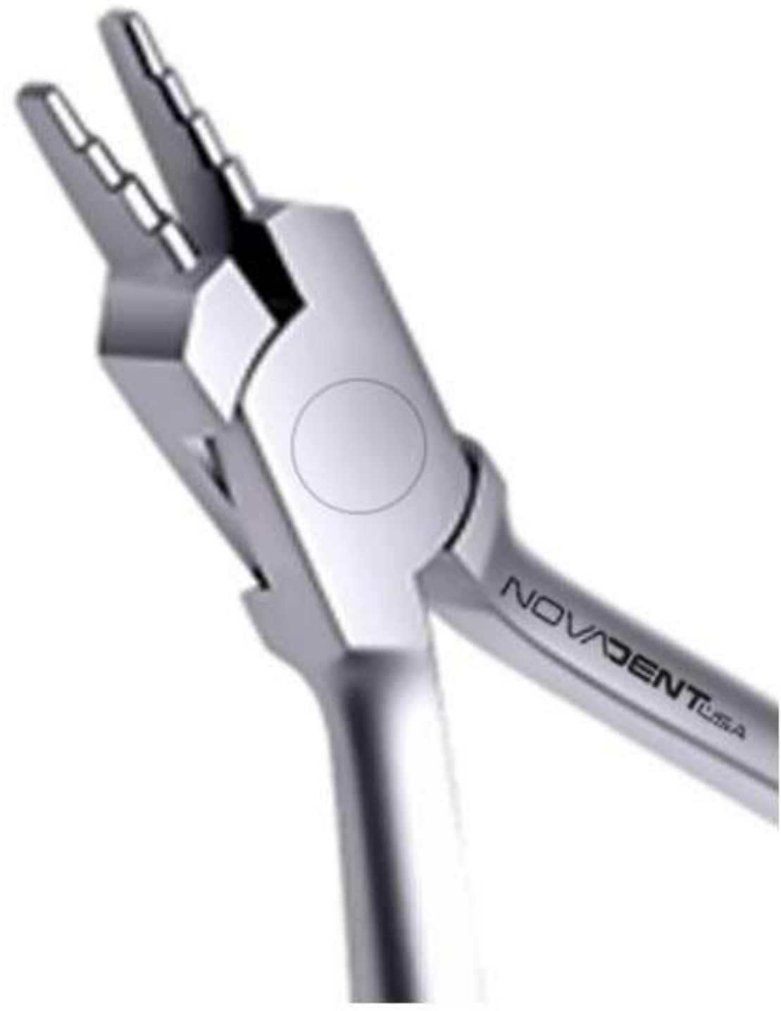
NANCE LOOP FORMING PLIERS Four step beak to create 3,4,5 and 6mm loop designed for all wires upto 0.022"/0.56mm 2484
